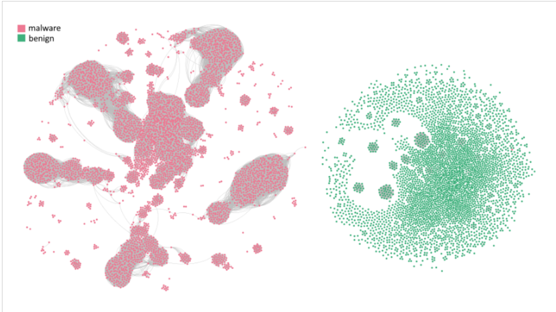
Figure 2.1: Illustration of a similarity graph of a set of binaries. Each vertex represents a binary, and an edge connects two vertices if the corresponding files exhibit similarity based on a specified similarity measure. In this specific illustration, the files are considered similar if their TLSH difference score is below the threshold of 40. Malware binaries are denoted by red nodes, while benign binaries are depicted as green nodes. Notably, there is a clear distinction between malware and benign files, and the similarity graph of malware exhibits significant clustering.
